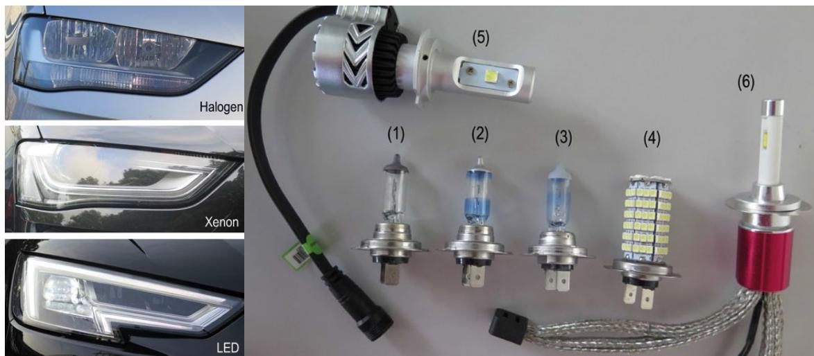
Slika br. 1 – Vrste farova odnosno sijalica u ispitivanju: (1)Osram original 64210-01B, (2)Osram Night Breaker Unlimited, (3)Philips WhiteVision Xenon-Effekt, (4)Carchet LED, (5)Neverland LED, (6)Car Rover LED
